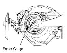
The overdrive clutch pack clearance should be set at .022" to .047" (0.55mm – 1.20mm). Measure using a feeler gauge between the top pressure plate and the selective snap ring. To achieve the recommended clearance, use one of the selective snap rings available from local Ford dealer.
