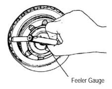
Apply air to assembled clutch pack several times to seat the friction and steel elements. Using a feeler gauge measure between the bottom of the selective snap ring and the top of the pressure plate. Clearance should be .040" to .075" (1.02 to 1.91mm). Adjust clutch pack clearance by selecting the correct selective snap ring.
