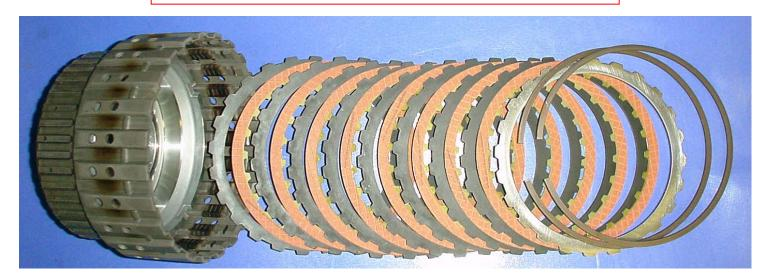
Alto received several requests from builders around the world to produce a PowerPack® that provides more capacity for the Direct clutch of the RE5R05A transmission. Now you can replace the 5 friction elements with 7 friction elements and the 6 friction elements with 8 friction elements in the Direct clutch drum of this unit.
