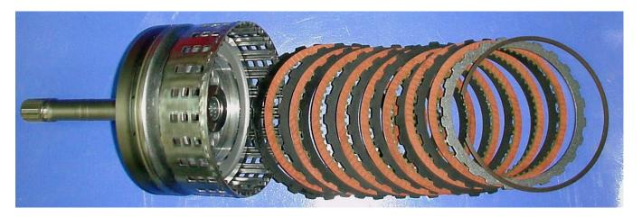
Alto received several requests from builders around the world to produce a PowerPack<sup>®</sup> that provides more capacity for the Input clutch of the RE5R05A transmission. Now you can replace the 6 friction elements with 7 friction elements and the 7 friction elements with 8 friction elements in the Input drum of this unit.
