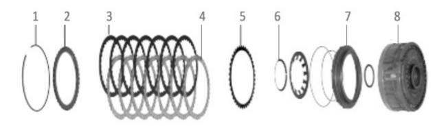
**Installation:** Stack the 2-6 brake (Intermediate) clutch pack as follows:
