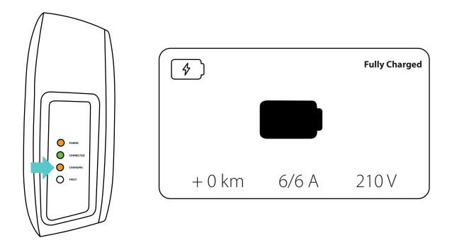
6. Disconnect the charger when the charge is completed by pressing the release button on the Charge Coupler and removing it from the vehicle.
