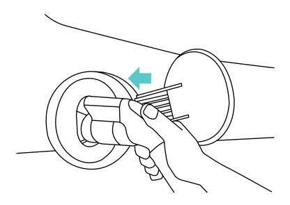
4. Charging begins automatically. Power will be delivered in accordance to the demand of the vehicle. While chaging, the Charging Indicator will blink continuously. Always verify that the vehicle charging status indicator by checking your vehicle panel.
