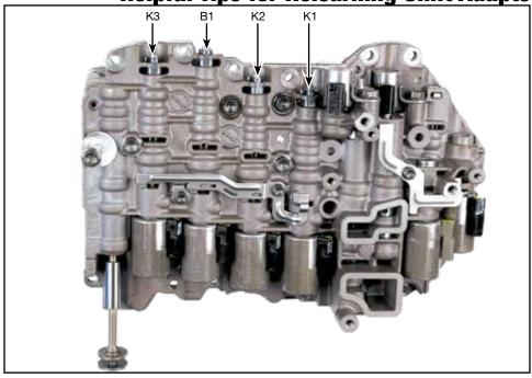
The 09G is an adaptive learn transmission. After transmission overhaul, replacement or valve body replacement, the shift adapts must be cleared to zero and then the vehicle must be driven for the TCM to relearn the new shift adapts.
