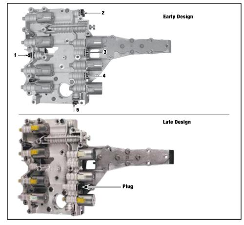
5R110W solenoid body **F05R110** is serviced without any pressure switches. Your original solenoid body may have one or five pressure switches depending on model year. The computer on these vehicles was never programmed to monitor the pressure switches and Ford removed them in late 2004. The later solenoid body may have one pressure switch with no wire going to it. In this application it is only used as a plug with the remaining four holes cast over.
