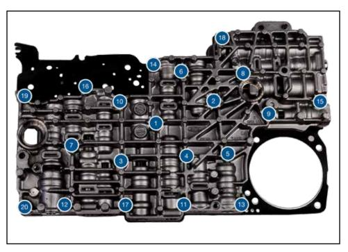
Torque valve body bolts in sequence shown: 89 in-lb
