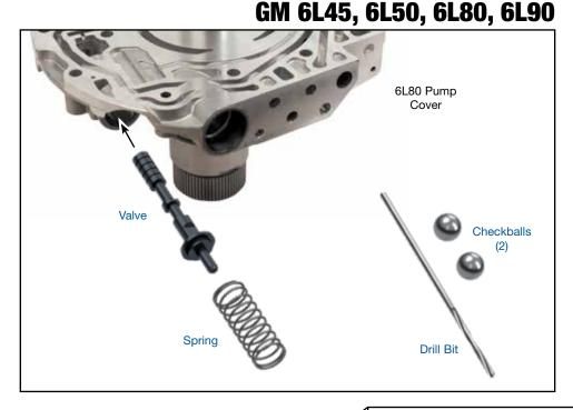
**NOTE:** In GM 6L45, 6L50, 6L80 and 6L90 units the pressure regulator valve and boost assembly are located in the pump cover. Transmission must be removed from the vehicle to access pump and replace the pressure regulator valve.
