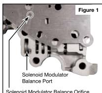
Solenoid Modulator Balance Orifice Drill with .062" bit. Insert .062" aluminum plug into orifice and peen shut.
