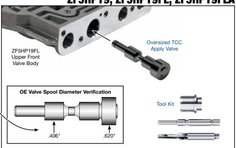
**NOTE:** The valve body section incorporating the TCC apply bore also has three other valve bores. Removal of the end plate will release the valve trains from all four bores. Recommend removing each valve train to thoroughly clean valve body after completing the reaming process. Ensure valve train components do not get mixed or misplaced during this process.
