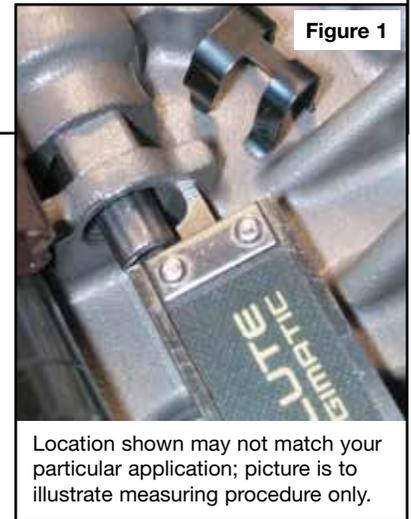
**CAUTION:** Prior to the removal of any control valve adjustment plug, measure and record the distance from the plug to the casting. This measurement must be duplicated upon assembly (**Figure 1**).
