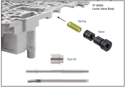
CAUTION: Prior to removal of spring adjustment plug, measure and record the distance from the plug to the casting (Figure 1). This dimension must be matched during reassembly.
