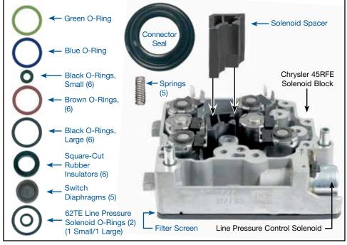
NOTES AND CAUTIONS: Care needs to be taken to ensure that there are no misplaced solenoids when working on these units. Chrysler uses two different solenoid designs housed inside of this solenoid assembly. These are:
