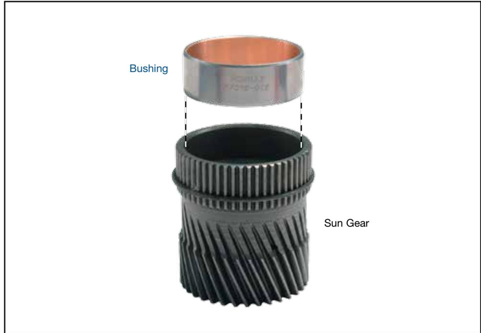
Install bushing using arbor press.
