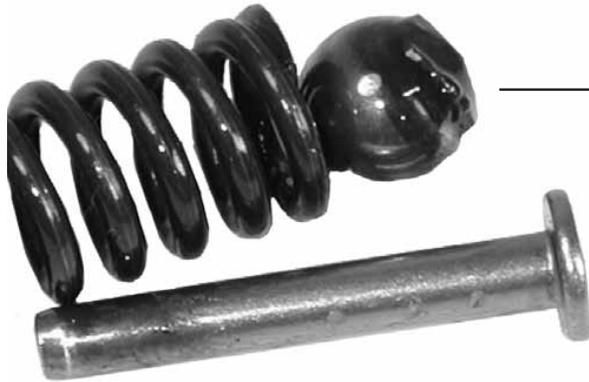
Remove the relief rivet and clean ball and seat. With severe contamination, reform the seat by tapping ball into it.
