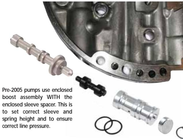
Pre-2005 pumps use enclosed boost assembly WITH the enclosed sleeve spacer. This is to set correct sleeve and spring height and to ensure correct line pressure.
