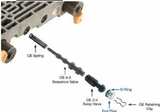
21. Replace end plug with O-ring end plug provided.
