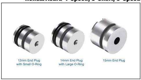
**NOTE:** Sonnax end plugs fit bores with 12mm, 14mm or 15mm OE end plugs. It is necessary to measure OE end plug diameter to verify compatibility with a particular bore. Recommend installing end plugs in following bores: CPC A, CPC B, Shift Valve C, L/U Shift, L/U Control.
