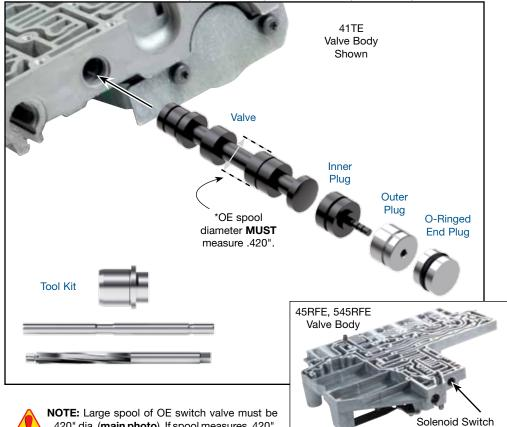
NOTE: Large spool of OE switch valve must be .420" dia. (main photo). If spool measures .420", continue installation. If spool measures .453", STOP! This Sonnax kit cannot be used.
