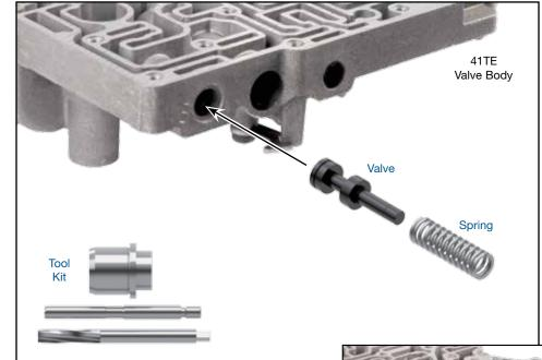
CAUTION: Spring will shoot out of bore during retainer clip removal. A flat-blade screwdriver can be used to hold spring while removing retainer clip.
