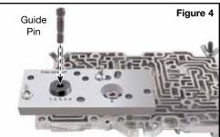
Securely tighten wing nuts on jig plate, holding all components together, while letting Sonnax guide pin move freely in OE accumulator bore.
