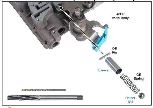
NOTE: Never reuse OE detent ball with Sonnax sleeve. The Sonnax replacement ball is specially toleranced to work with this sleeve and prevent binding of the ball in the bore.
