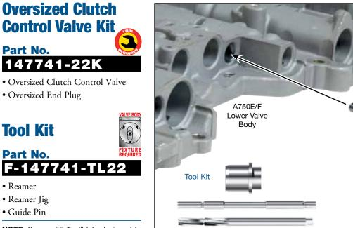
NOTE: Sonnax "F-Tool" kits designed to service a specific bore require the VB-FIX, a self-aligning valve body reaming fixture. More information and instructions can be found online at www.sonnax.com.
