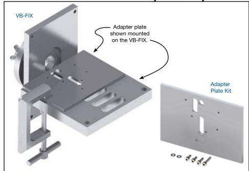
**NOTES & CAUTIONS:** Adapter plate kit **F-15741-TL29PL** is required to help secure small valve bodies to the **VB-FIX**. If you do NOT have these six designated screw holes (see above) on your adapter plate, you have an early-style with four designated screw holes. This early-style adapter plate must be modified for the AW55-50SN application. Directions on how to do this are located on page 2.
