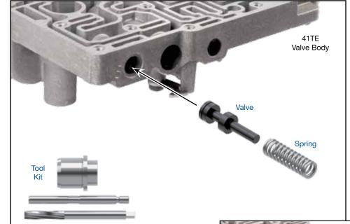
CAUTION: Spring will shoot out of bore during retainer clip removal. A flat-blade screwdriver can be used to hold spring while removing retainer clip.
