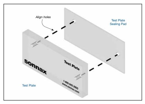
**NOTE:** Sonnax test plate sealing pads are intended to be used on clean, dry surfaces. Oil and debris will degrade pad over time, causing discoloration, deformation and/or nicks and tears. The pad should be rinsed in water to remove surface dust and debris. If contamination eventually renders pad unusable, discard and replace with new pad.
