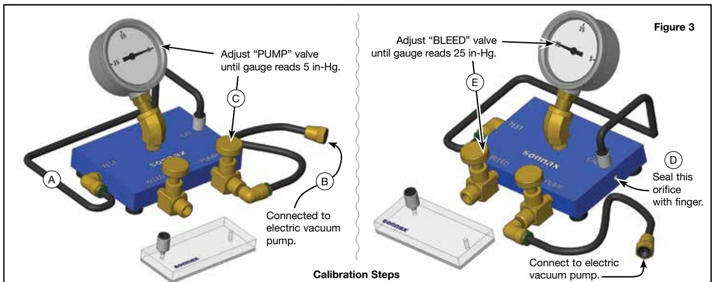
The test stand is now calibrated for repeatable results. Disconnect the non-flared flexible tube from the "CAL" fitting and insert it into the test plate push-to-connect fitting.
